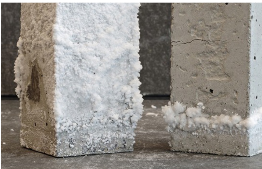
Extreme example of efflorescence on concrete block in a laboratory test.
