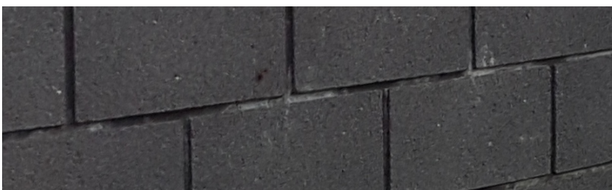
Picture, centre: Artificial efflorescence on concrete bricks. Picture, bottom: The same bricks after weathering for 1 year.
